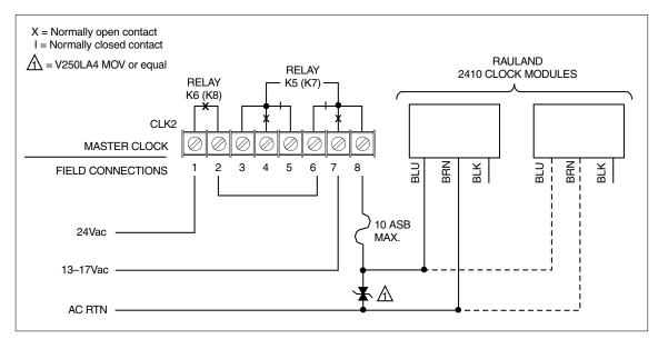
Figure B-11 Wiring Rauland 2410 Digital Clocks for 24Vac
